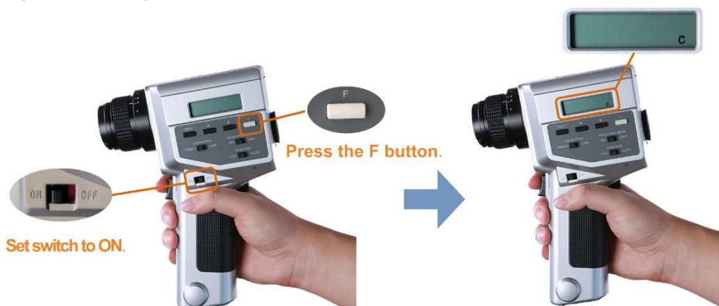
Figure 12-10 Setting CS-100A colorimeter
