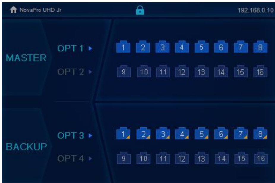
Figure 4-3 Optical fiber port statuses – Hot backup
