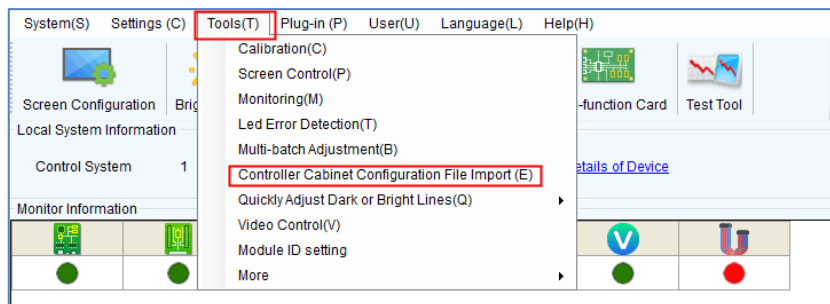
Figure 5-6 Importing controller cabinet configuration file
